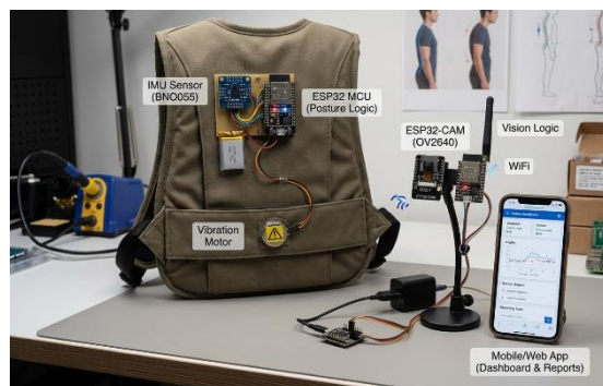
Figure. 3: Proposed Posture Corrector (a) framework and (b) component positioning.
